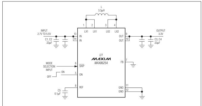
Figure 4. Typical Application Circuit (Fixed 3.3V Output)
