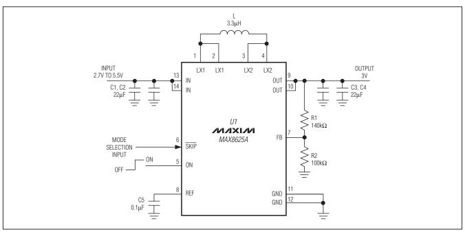
Figure 3. Typical Application Circuit (Adjustable Output)
